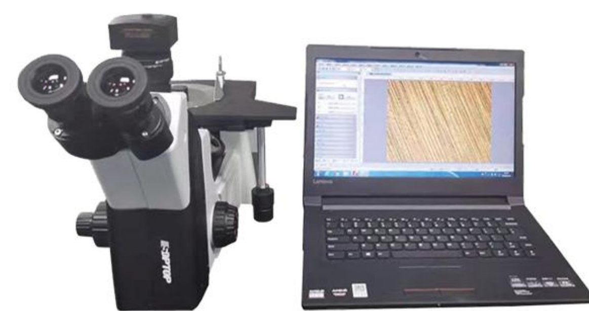
Coating thickness measurement
